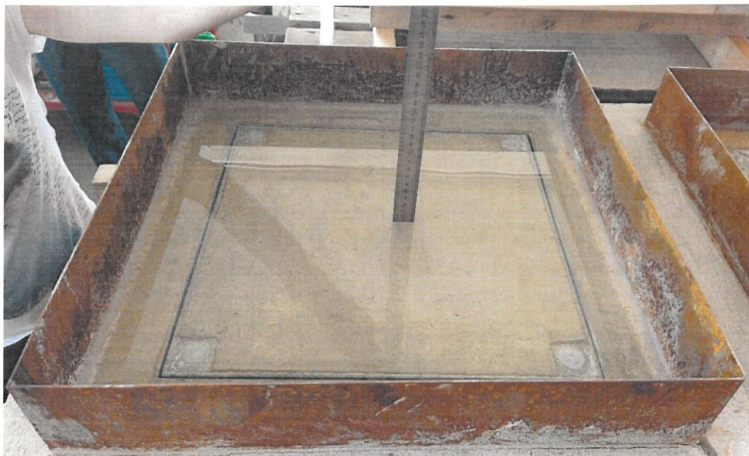
Figure 1: Watertightness test set up - ACO Access Cover UNIFACE 300x300x70, EI120
